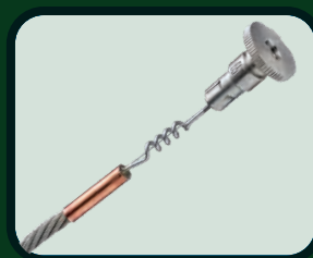
TYPE T EXPULSION FUSE 1 to 200 A. Fuse element material: Tin or silver alloy. Speed ratio: 10 to 13.1.
